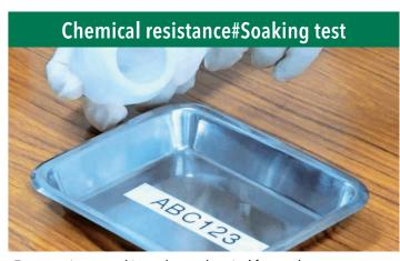
Tape was immersed in each test chemical for two hours.
